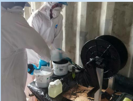
Figure 3: Kevlar tape impregnation with resin using BOBiPREG
