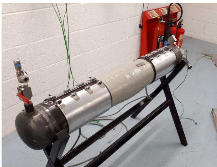
Figure 2. Energy release rate – qualification of R4D system at high temperature.
