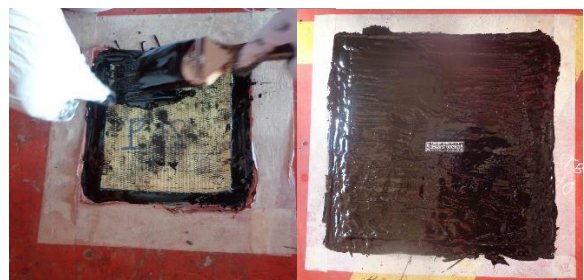
Fig. 5&6: Impregnation of the 2 nd patch and reference plate
