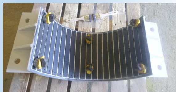
Figure 4: ROLLERKIT® fixing on support using magnets
