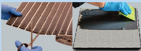
Fig. 2 & 3: Cutting the required quantity of ROLLERKiT pads and F3X8 filler application (illustrating pictures only)
