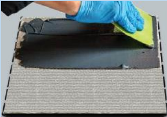
Figure 8: F3X8 filler application on ROLLERKIT® (illustrating picture only)
