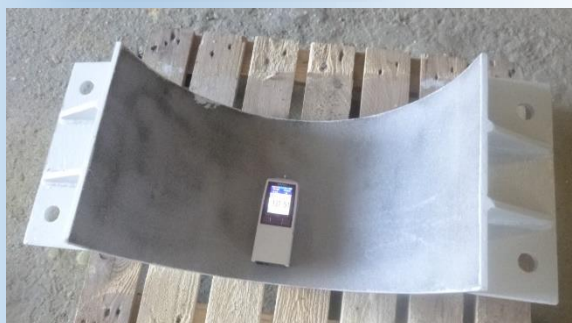
Figure 1: Roughness measurement on support sandblasted
